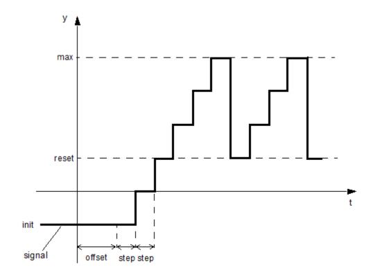
If the initial time offset is specified, the block outputs the initial signal value *init* until the simulation time reaches the *offset* value, at which point the counting cycle starts. The block outputs the current value for one time step, then repeatedly increments the signal value by 1 and outputs it for one time step, until it reaches the maximum value *max*. The block outputs the *max* value for one time step, then returns to the *reset* value, and the counting cycle starts again.
