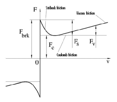
The Stribeck friction,  $F_S$ , is the negatively sloped characteristics taking place at low velocities (see [1]). The Coulomb friction,  $F_C$ , results in a constant force at any velocity. The viscous friction,  $F_V$ , opposes motion with the force directly proportional to the relative velocity. The sum of the Coulomb and Stribeck frictions at the vicinity of zero velocity is often referred to as the breakaway friction,  $F_{brk}$ . The friction is approximated with the following equations:
