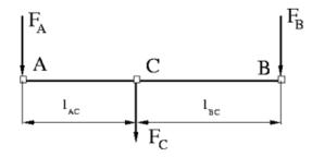
The summing lever equations are derived with the assumption of small angle deviation from initial position:
