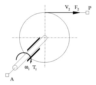
The wheel and the axle have the same axis, and the axis is assumed to be rigidly connected to the frame, thus making this mechanism an ideal converter of mechanical
